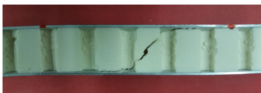
Fig. 4c. core fracture (PSP 2)
